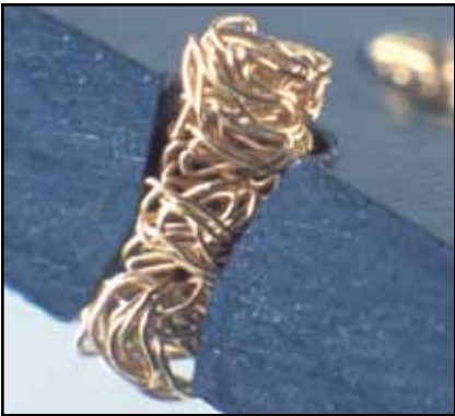
Connector Cross Section Showing CIN::APSE® Contact
