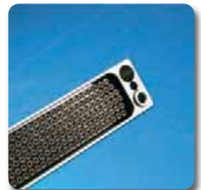
High density metal shelled PCB and LRM with flex
