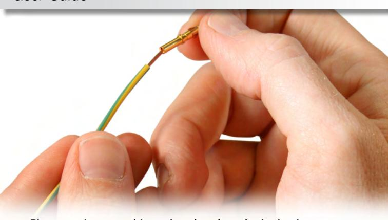
Place conductors, with no deteriorations, in the bucket contact.
