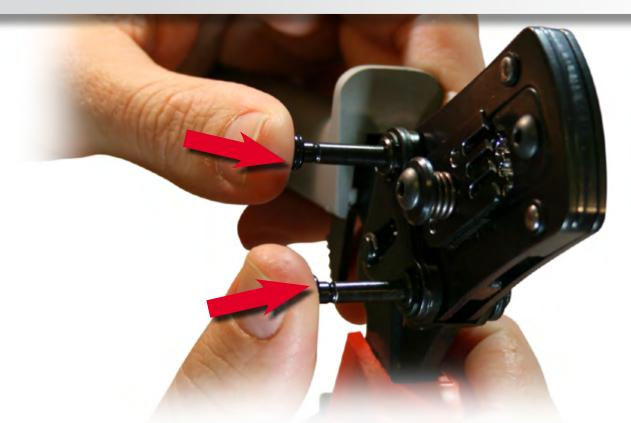
Close simultaneously the two pins to maintain the head.
