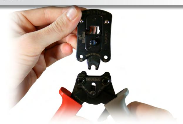
Choose the adapted head, keep vertically and slide it into the handle till the mecanical end.
