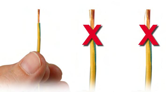
Strip the cable properly checking the size recommended in the catalog.
