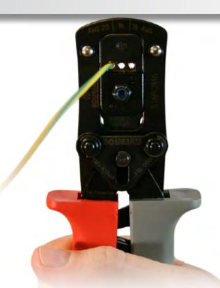
To crimp contact assembly-cable, tighten sharply the clip to the end of the mechanism.
