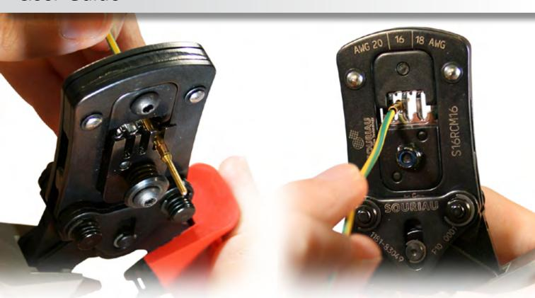
Position the contact in the bottom of the tools by checking out its orientation.
