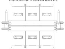
This drawing shows an installation example. In an arrangement of multiple high power modules electrical data can differ from the single module.
