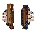
Designed for through panel mounting disconnect for harsh environments; Quick Install has many functions in one single piece: mating effort reduction thanks to 4 ramps designed to bring a "gearing down" function; specific material with low friction coefficient, various inserts type and screw washer for fixing process.
