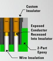
Cinch's unique plug insulators are designed to provide increased electrical protection between contact cavities preventing any potential shorts due to exposed wire or epoxy voids. Comprised of PEEK material these connectors offer superior performance and long life in severe environments.
