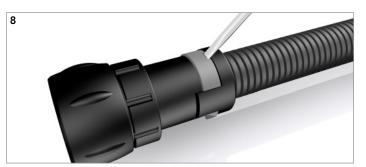
To release the locking mechanism, use a screwdriver.
