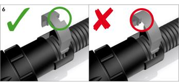
Take care of the oval retaining clip orientation and locate it in the slot provided.
